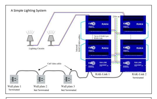
This picture shows a simple lighting installation using the Rako Wired system.
