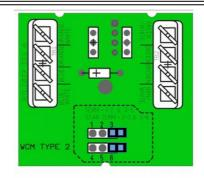
NOTE: Devices are supplied unterminated with jumpers in positions as above
