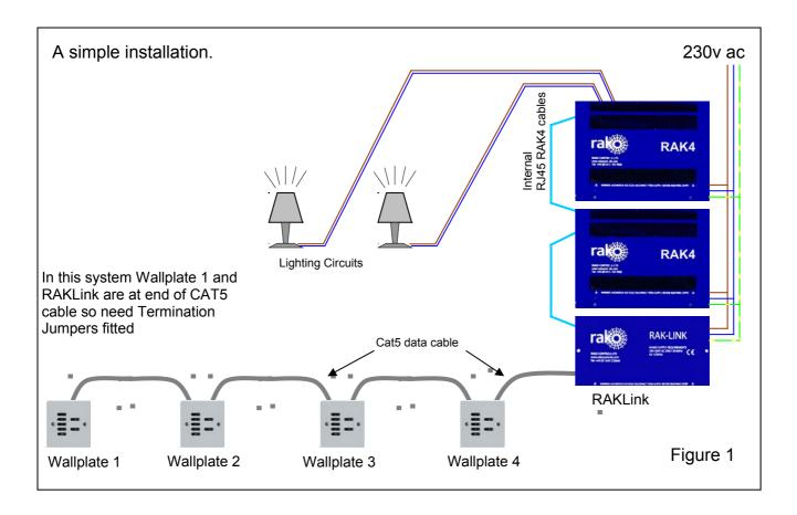
Figure 1 shows a simple lighting installation using the Rako Wired system.
