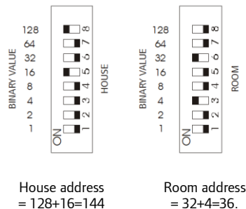
Fig 3. Addressing Switches
